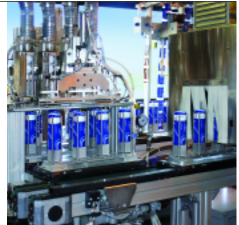
A custom-made automatic ball inserter drops balls into sleeves just ahead of the shrink tunnel.
