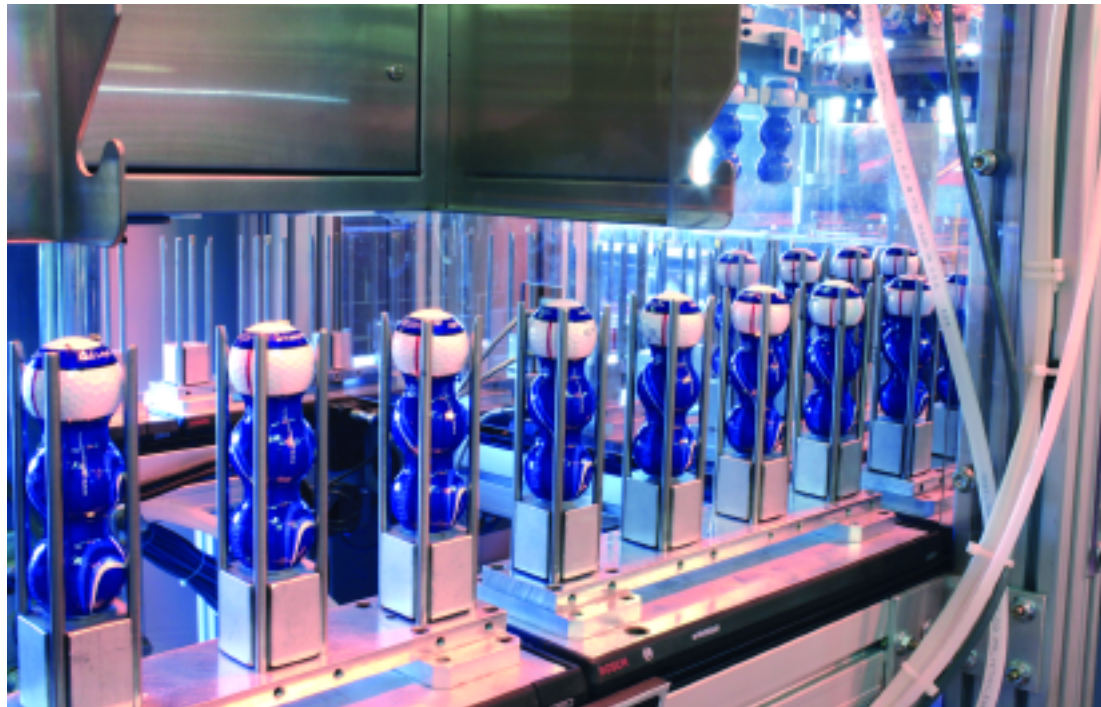
Shown here are the four-station conveyor pallets emerging from the shrink tunnel. Each station holds three shrink-sleeved balls.
